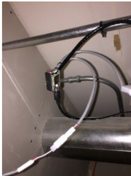
The two grey wires go through the wall, down the frame, and to the two door switches (via Molex connectors for easier maintenance), the lower black cable is power from a USB wall wart, and the upper black cable goes to the indicator lights—more on that later)
